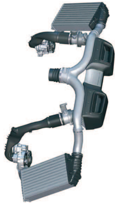
Fig.25: Air cleaner, air ducts, intercoolers
