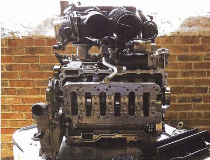
Combined cylinder bank/outer crankcase casting (top, left) was chosen to simplify the manufacturing process. Connecting rod (top, right) for a 3.4-liter 996 engine; piston is dished for the four-valve heads. Partially disassembled 996 engine seen in profile, with the iron main-bearing saddle clearly evident (above, left). Another view of the main-bearing saddle (above, right). Four-valve 996 cylinder head (left) showed little wear after 100,000+ miles, though the chain ramps for the 996's VarioCam timing system did show their age...
