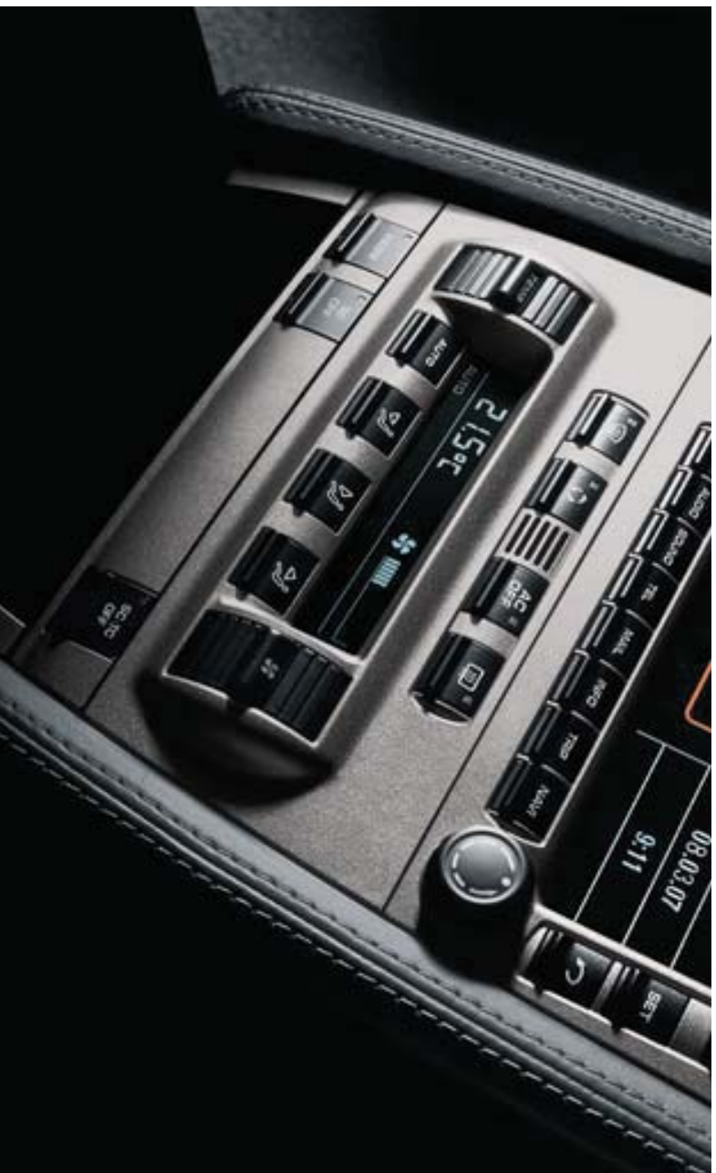
Fig. 21: SC OFF and SC+TC OFF buttons in the control panel/center console
