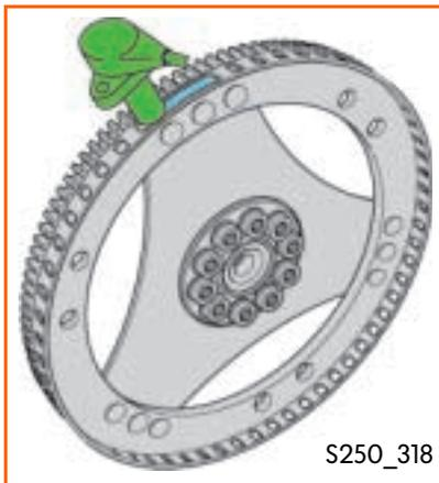
Engine speed sender G28 provides an important input signal. It is located in the gearbox housing.
