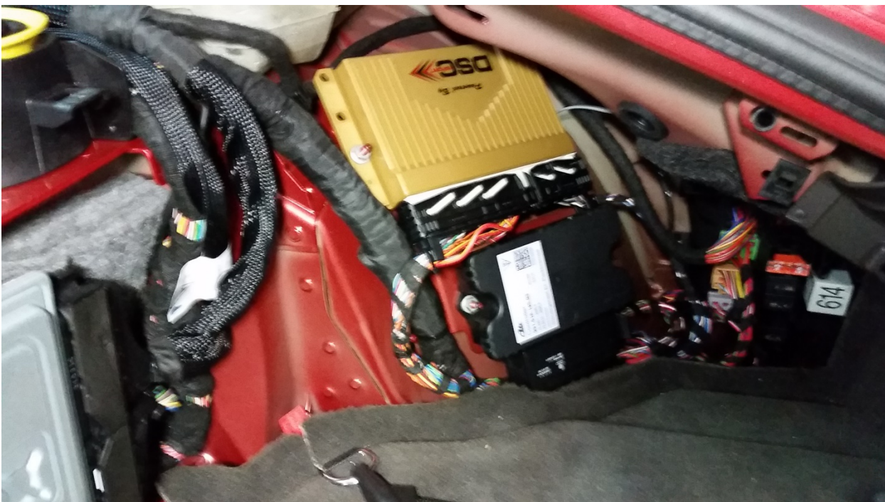
Figure 6-2. DSC unit fully mounted in place
