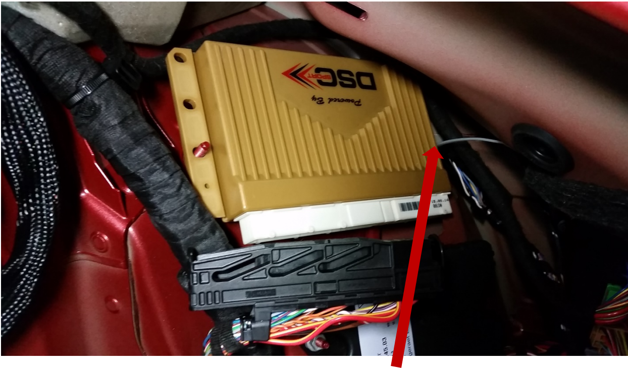
Figure 6-1. DSC module fit in place with cable-tie holding right-side.
