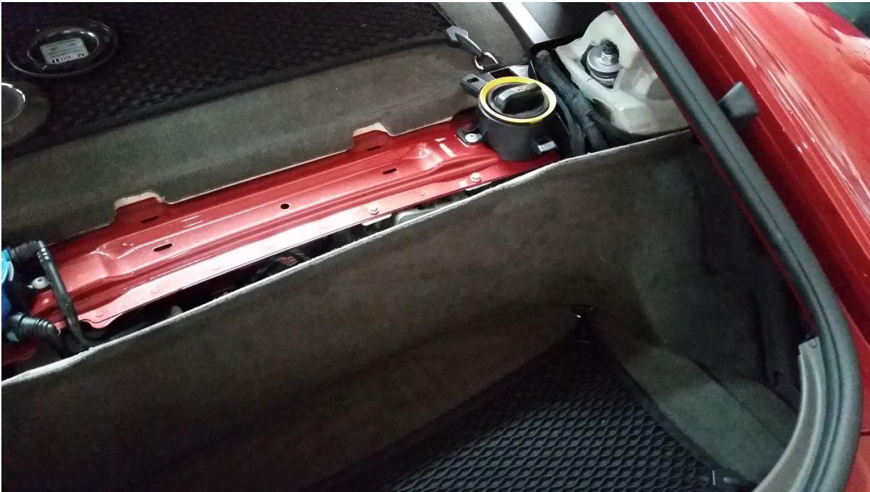
Figure 4-1. Engine bay carpet section before removal
