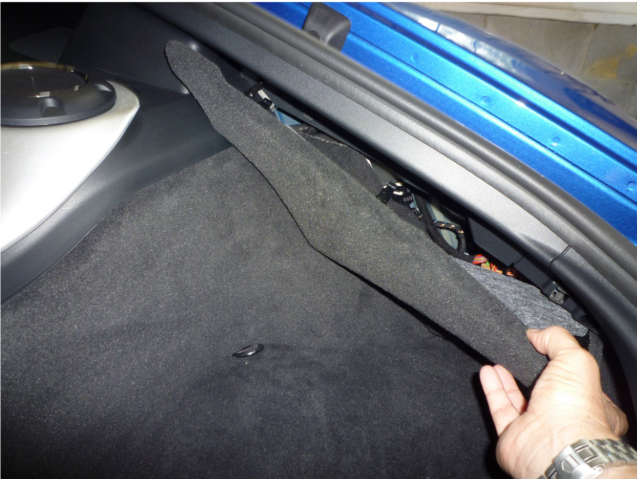
Figure 1. Rear Side Carpet removal
