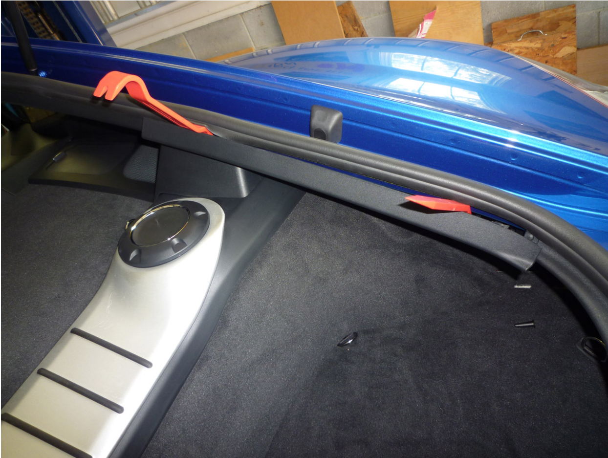
Figure 2. Side plastic trim removal
