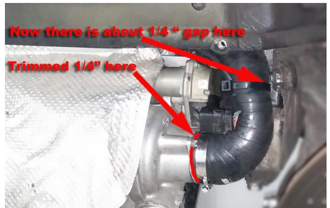
It is possible the hoses rub against the body. If so, you can trim them as indicated.
