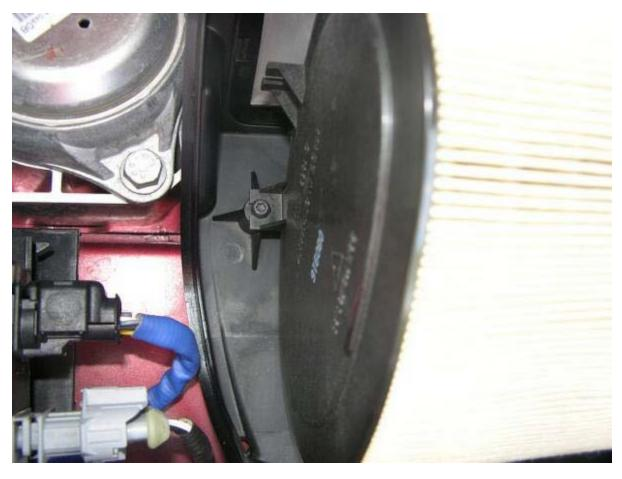
Once the screws have been removed, grab the filter at the end and gently wiggle it off of the mount.
