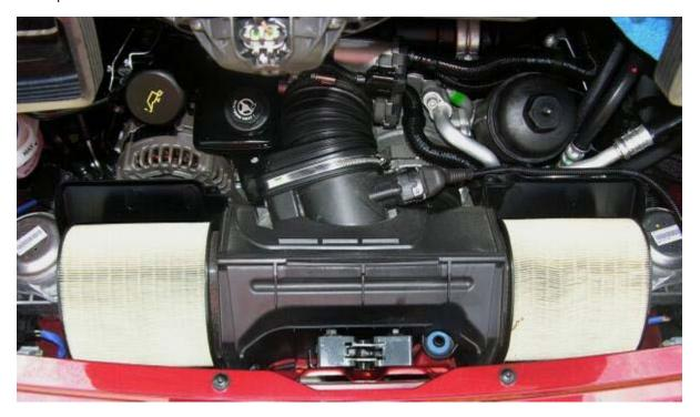
Each filter is held at the end with a Torx screw which can be removed with a T20 driver
