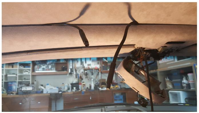
The power cable is only about 3/16" and no large connectors so the wiring was done in a snap. The mirror can get input from two sources, with the primary source using the reverse light voltage to trigger the screen on, so it is easy to wire this into the trigger for the camera. I have also installed a wireless feed for a front camera that I have not installed yet.
