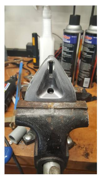
I used a little epoxy glue and a bolt to hold the mount and mirror together
