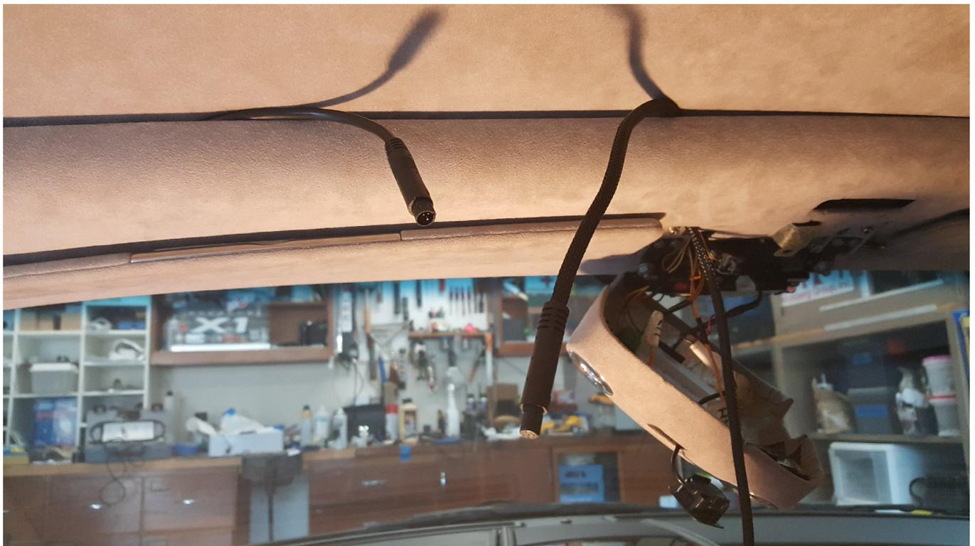
The power cable is only about 3/16" and no large connectors so the wiring was done in a snap. The mirror can get input from two sources, with the primary source using the reverse light voltage to trigger the screen on, so it is easy to wire this into the trigger for the camera. I have also installed a wireless feed for a front camera that I have not installed yet.
