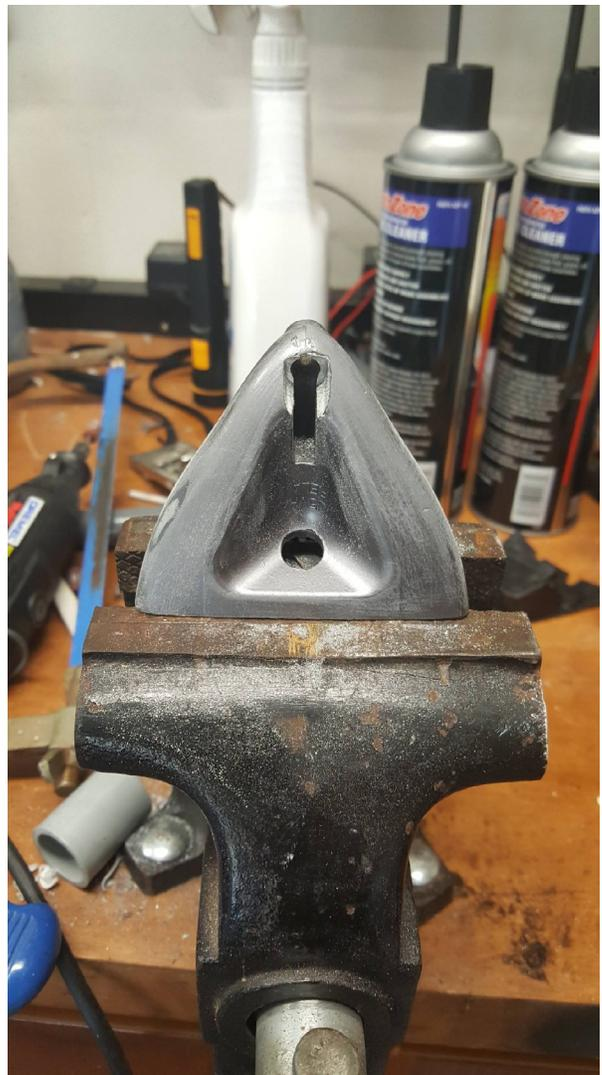
I used a little epoxy glue and a bolt to hold the mount and mirror together
